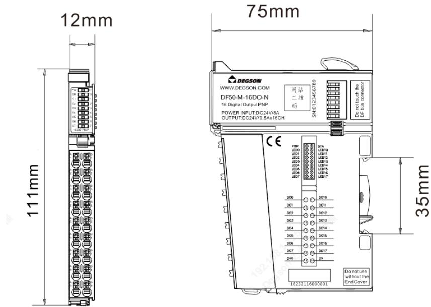
16 channel digital output /24VDC/NPN
