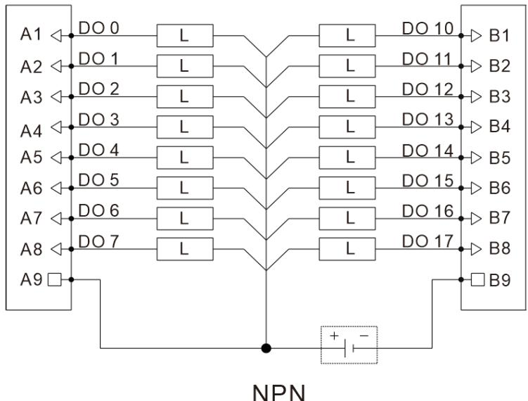
Note: A9 and B9 24V power supplies are provided externally.
